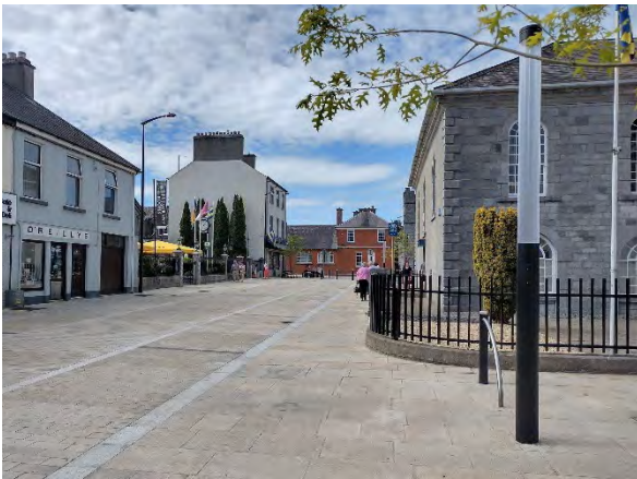
Roscommon Town Square. Note the lack of kerbs and presence of bike parking infrastructure.
