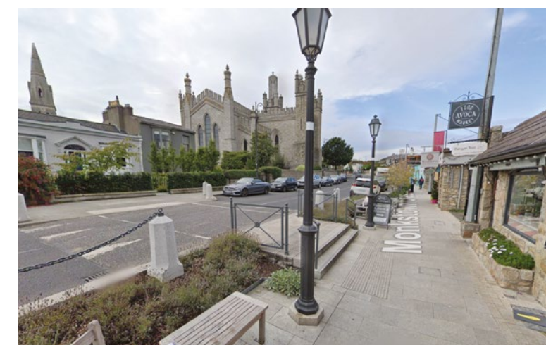
Illustration used in DMURS showing high quality material, planter buffers between road and paths, Monkstown Crescent, Co Dublin
